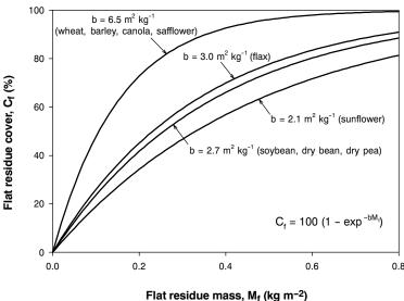
Figure 4. Relationship in WEPS to calculate flat residue cover from flat residue mass for the nine crops in this study. A flat residue mass of 0.2 kg m<sup>-2</sup> provides about 35% cover for soybean, dry bean, and dry pea. The same mass provides about 70% cover for wheat, barley, canola, and safflower.
