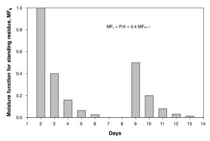
Figure 2. Behavior of the moisture function for standing residue  $(MF_s)$  if precipitation were equal to or greater than 4 mm on day 2, equal to 2 mm on day 9, and all other days were dry. In this example, moisture is optimum for decomposition on day 2, 40% of optimum on day 3, etc. No decomposition occurs on days 1, 7, 8, and 14 because of a lack of moisture. For flat residue, not only precipitation, but also surface soil water content affects decomposition
