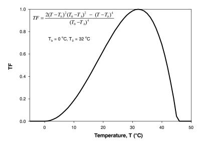
Figure 3. Plot of the temperature function (TF). Temperature is optimum for decomposition at 32 °C. Below 0 °C and above 46 °C, no decomposition occurs.
