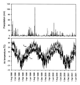
Figure 5. Daily precipitation, maximum air temperature  $(T_{\rm max})$ , and minimum air temperature  $(T_{\rm min})$ , measured at the Area IV Soil Conservation Districts USDA-ARS Research Farm near Mandan, North Dakota, used to drive the WEPS decomposition model.
