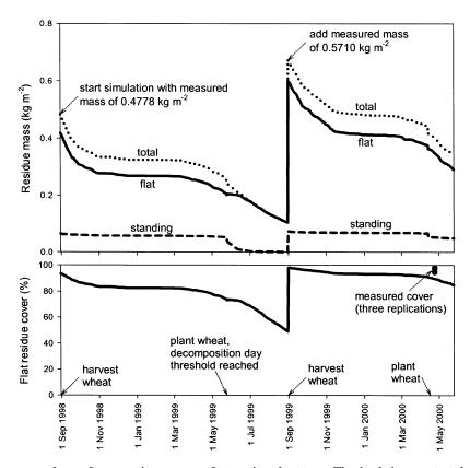
Figure 7. Simulated residue mass and cover for a cropping sequence of two spring wheat crops. The simulation was started after the first wheat harvest with a measured residue mass of  $0.4778 \text{ kg m}^{-2}$ . After the second wheat harvest, a measured residue mass of  $0.5710 \text{ kg m}^{-2}$  was added to the existing residue pool. Measured residue mass is the mean of four replications.
